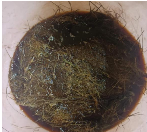
Fig. 2 Alkaline Treatment of fiber
